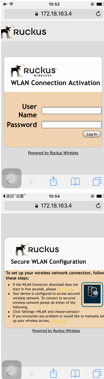
FIGURE 61 Activate device using the WLAN Connection Activation screen, and download activation file
