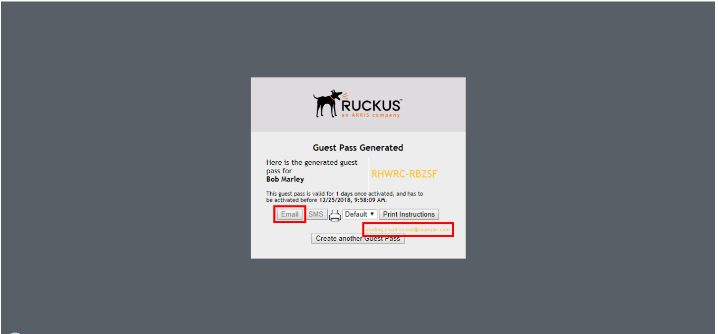
FIGURE 77 Click Email to send the guest pass key to the email entered on the Guest Information screen
